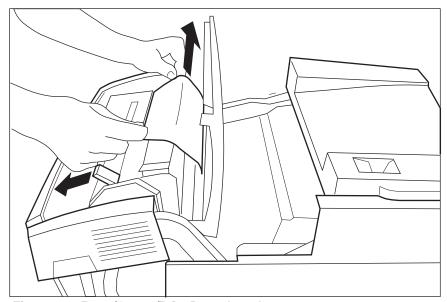
Figure 6-2: Fuser/Output/Print Drum Area Jam
